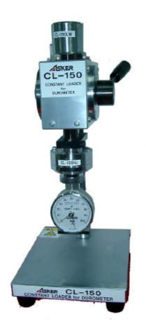
When attempting to measure hardness manually, inconsistent pressures and/ or speeds are used while pressing the indentor and presser foot. This causes a problem of deviation in measured results. To solve this problem, CL-150 Series constant pressure/speed loaders have been developed. Applicable standards refer to this type of loader as a 'Durometer Holder.'
