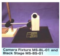
Convenient for viewing images up to A4 size. Then stage can be moved manually.
