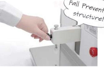
Jig is exchangeable by turning the front knob.
