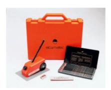
Using the same technique of evaluation with pencils as the Elcometer 3080, this instrument enables the pencil lead to be maintained at a constant force of 7.5N, and at the appropriate angle - which increases the reproducibility of the test.
